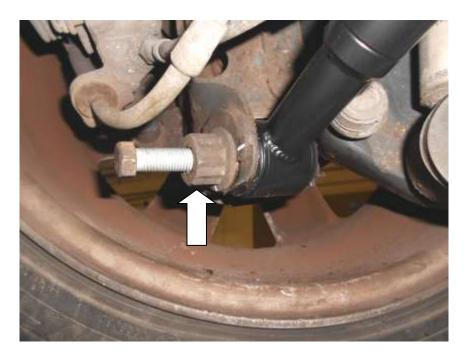
16. Using 24mm Ring-spanner rotate the snail cam adjuster into the position marked during disassembly. Using a 16mm socket and  $\frac{1}{2}$ " ratchet tighten the centre bolt and lock the adjuster in position.
