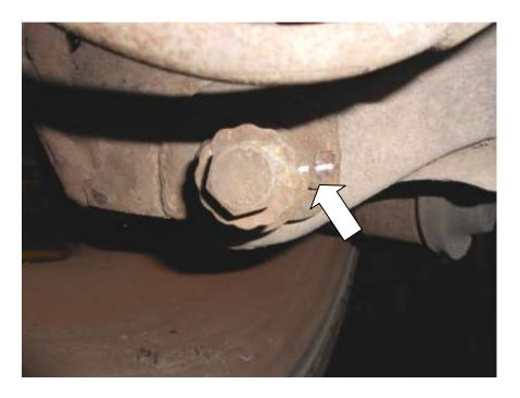
7. Using an 18mm socket, short extension bar, suitable ratchet and 18mm spanner undo the top bolt and remove it. Access is very restricted to get the 18mm socket on the head of the bolt.
