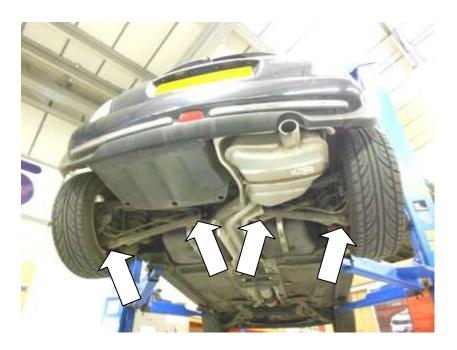
3. Support the weight of the rear wheel and suspension using a transmission jack or similar.
