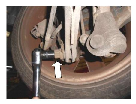
9. Place a piece of packing material between the lower part of the tie bar and the wheel. Pull the tie-bar downwards to release it.
