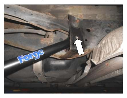
14. Push the wheel outwards to allow the other end of the tie- bar to push into position. You may need to undo one of the locking nuts to allow one end of the tie-bar to rotate if necessary.
